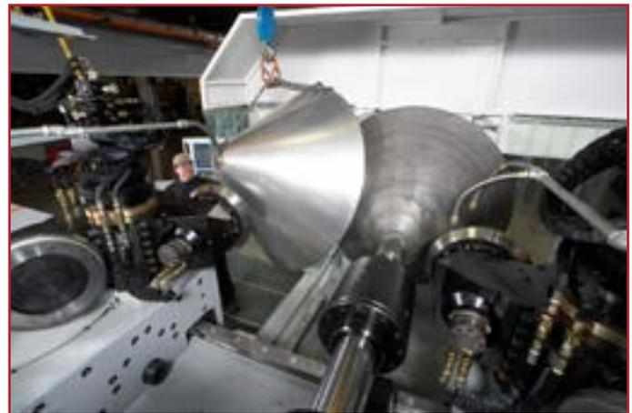
*Specializing in heavy gauge spin forming, Glenn Metalcraft manufactures components that are shaped from metal disks like the one pictured here.*
